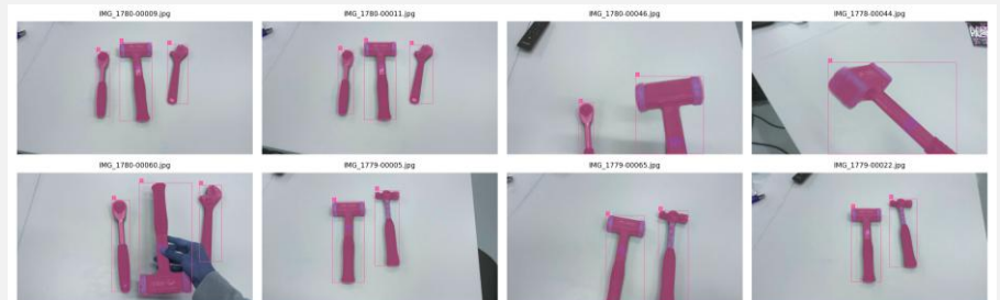
Figure 2. The model misclassifies all tools as hammer.
